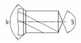
Solid carbide step drill, coated Shank DIN 6535 HB long 5x6,5/90°x28x6x90mm;Z2
