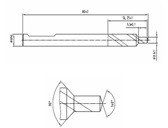
Solid carbide step drill, coated Shank DIN 6535 HB long 3x5,5/90°x25x6x80mm; Z2
