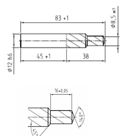
Solid carbide step drill, coated Shank DIN 6535 HA 8,5 x 16/90° x 12 x 83 mm, Z=2 8,5x90°x12x83
